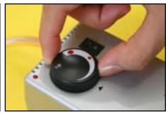
Switch on the apparatus by turning the regulators wheel. To warm up the apparatus, please leave the regulator for approx. 2-3 minutes on its lowest level.
